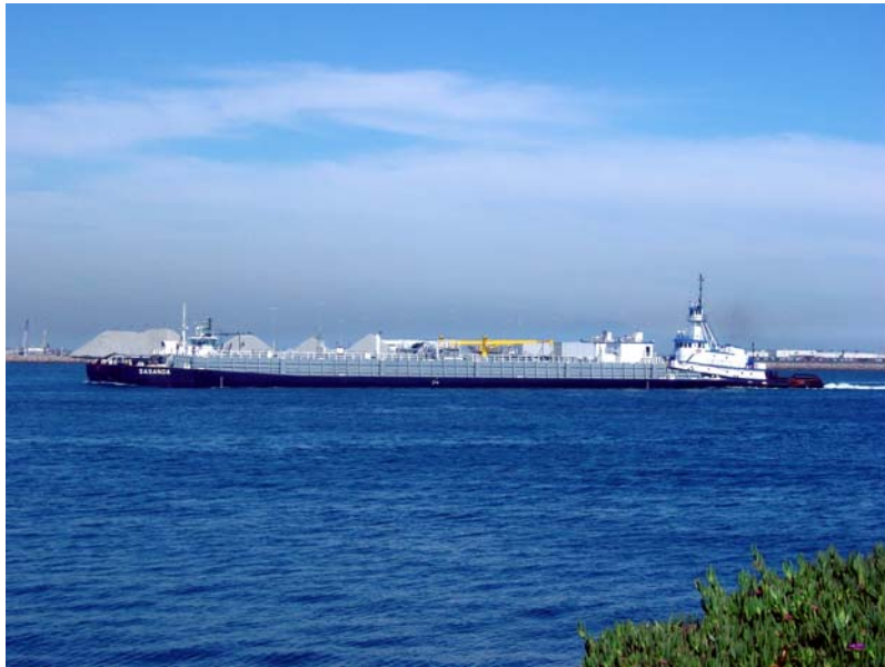
Figure 3.10: Integrated Tug and Barge
